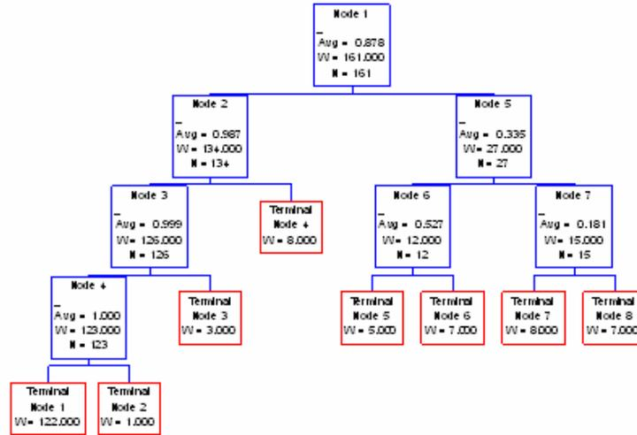
Figure 18. Constructed decision tree for leakage current approximation
