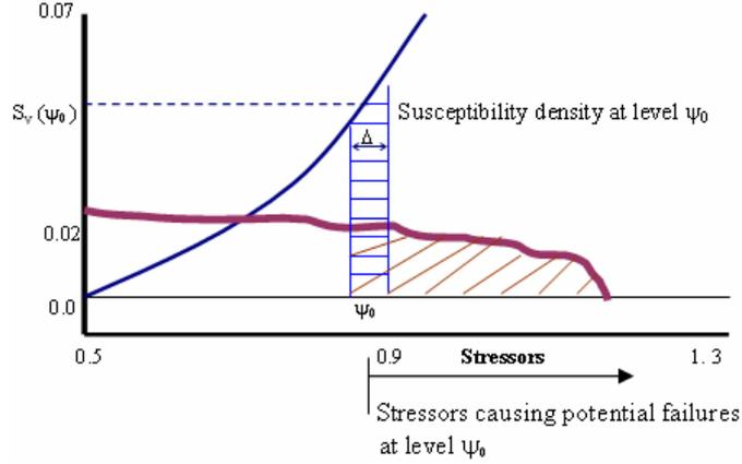
Figure 1. Stressor-Susceptibility interaction for single failure mechanism.
